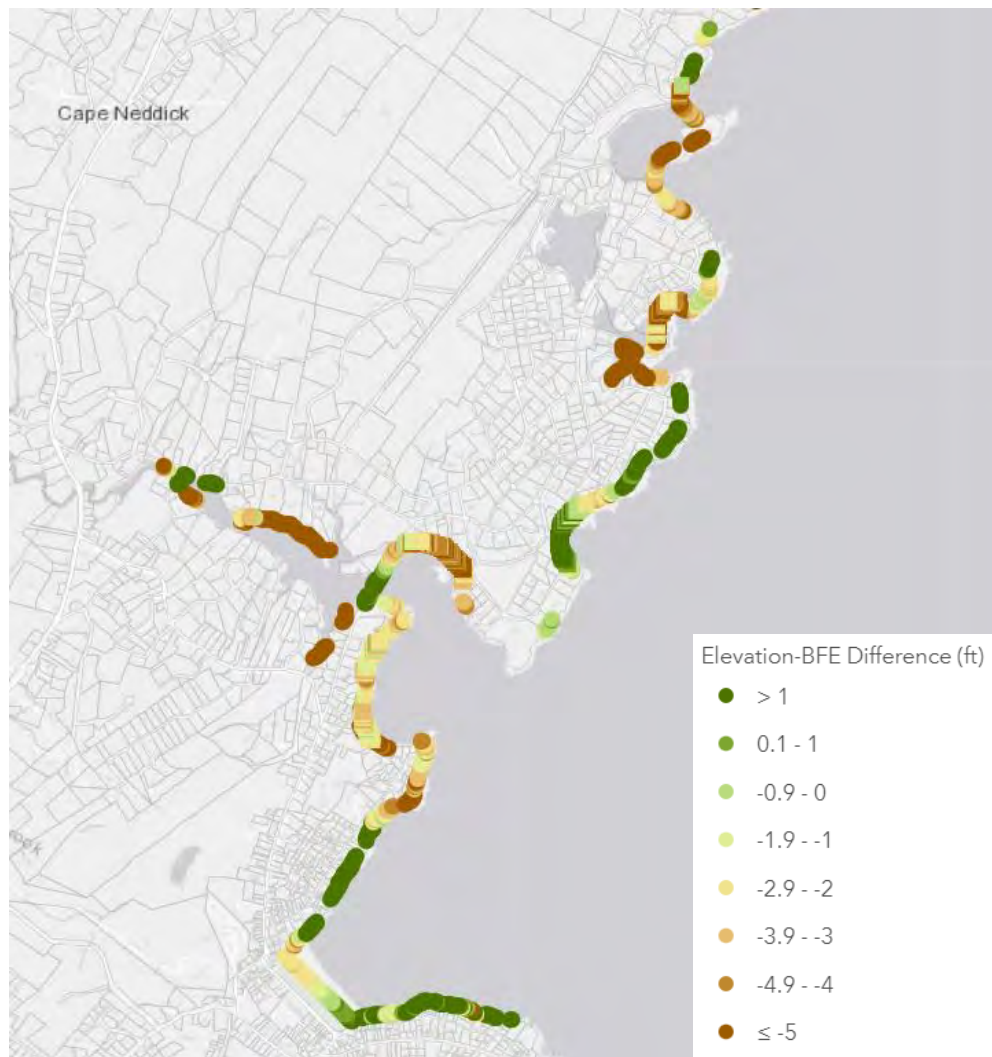
Figure 34. Coastal Engineering Structures (Circles) and Dunes (Squares) Elevation Above the 100-Year Flood BFE: Short Sands Beach, Cape Neddick River, and York Cliffs.
